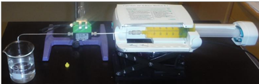
Figure 27 Setup of Flow Rate Dependency on the Syringe Plunger Level
