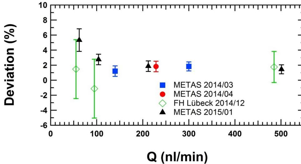
Figure 3 Calibration results at all flow points conducted by METAS and FH Lübeck.
