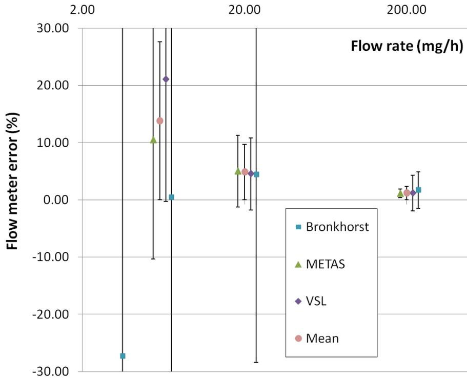
**Figure 5 Results intercomparison, close up of Figure 4. The uncertainty includes the uncertainty in reference flow rate, repeatability and the uncertainty due to drift. The indicated flow rate has been modified for visibility.**
