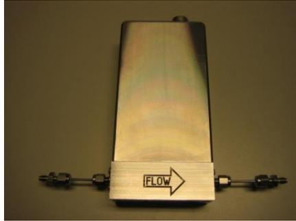
**Figure 1** Chip-based micro Coriolis mass flow sensor with 1/16" OD stainless steel tubes with an internal diameter of 125  $\mu\text{m}$  to connect the chip.
