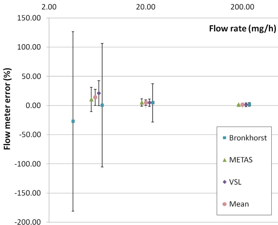
**Figure 4 Results intercomparison. The uncertainty includes the uncertainty in reference flow rate, repeatability of the calibration and the uncertainty due to drift. The indicated flow rate has been modified for visibility.**
