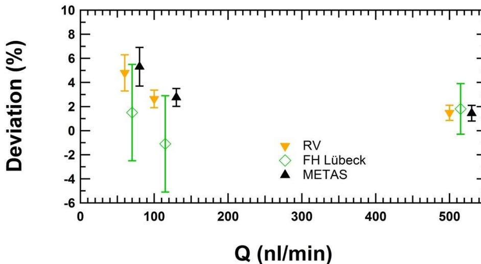
**Figure 6 Results intercomparison. The uncertainty includes the uncertainty in reference flow rate, repeatability of the calibration and the uncertainty due to drift. The indicated flow rate has been modified for visibility.**
