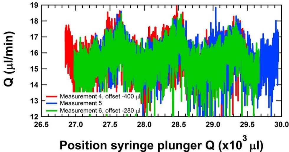
**Figure 25, DTI-Setup:** Instantaneous flow rates as a function of the position of the syringe plunger where a fit window of 3 s was used for the flow rate determination. 3 measurements were performed with the syringe (wet marked). The data are shifted with an offset in order to get an overlap of the pulsating flow pattern.
