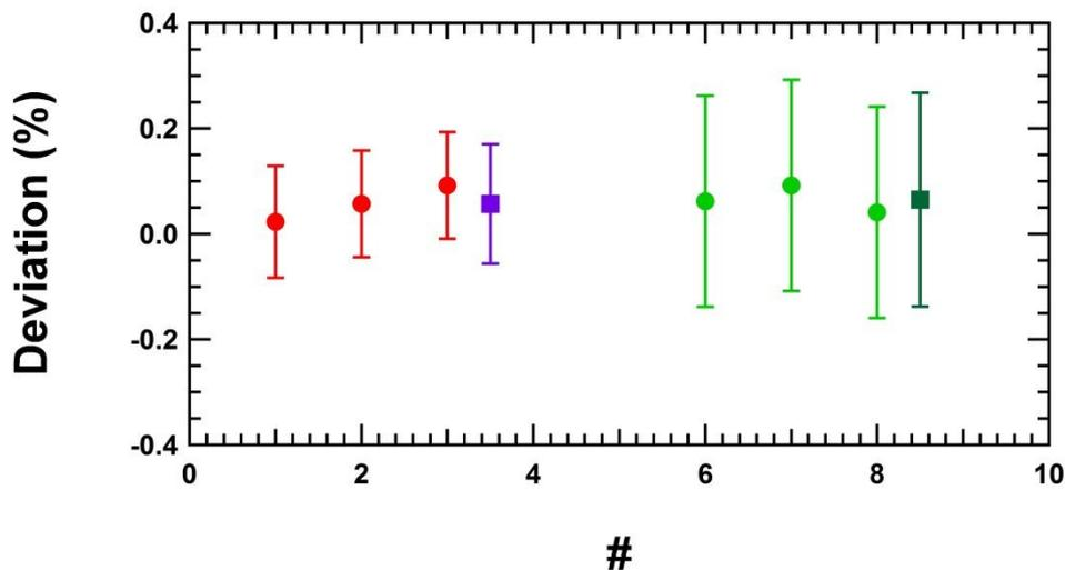
**Figure 21, METAS-Setup:** deviations of the M12P using the flow generator of the laboratory for stable steady flow (red circles) and the syringe pump for pulsating flow (green circles). The squares are the mean value of the 3 single points (circles).
