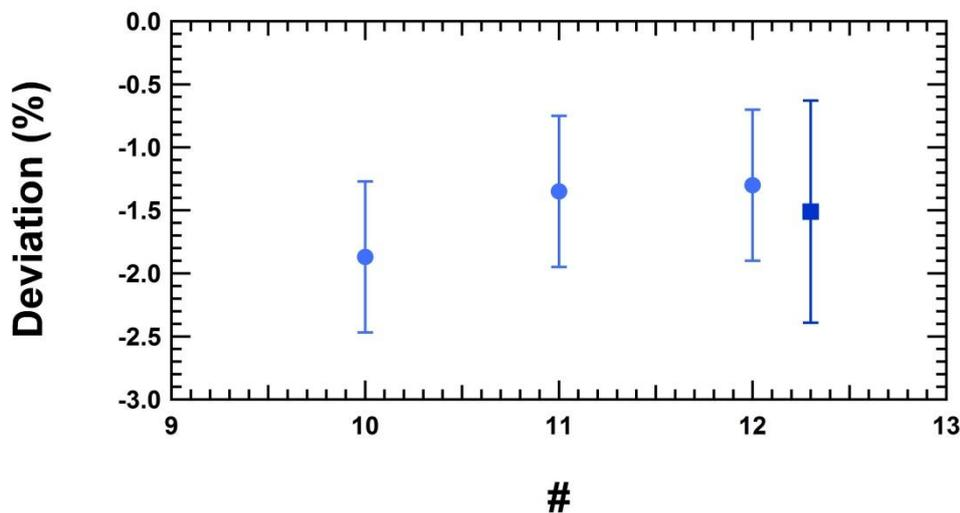
**Figure 13, METAS-Setup:** Deviations of the syringe pump using a wet syringe  $Q \sim 0.9$  ml/h (15.6 µl/min). The square is the mean value of the 3 single points (circles).
