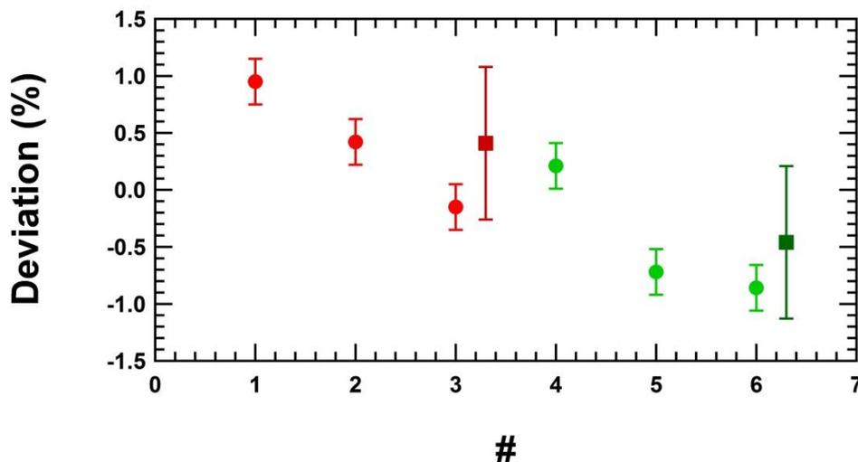
**Figure 10, METAS-Setup:** Deviations of the syringe pump using a dry syringe (dry marked, red circles) and a wet syringe (wet marked, green) at  $Q \sim 14$  ml/h ( $233 \mu\text{l}/\text{min}$ ). The squares are the mean values of the 3 single points.
