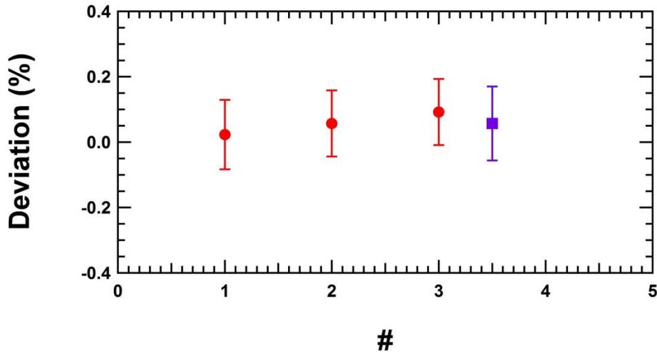
**Figure 16, METAS-Setup:** deviations of the M12P using the flow generator of the laboratory for stable steady flow. The square is the mean value of the 3 single points (circles).
