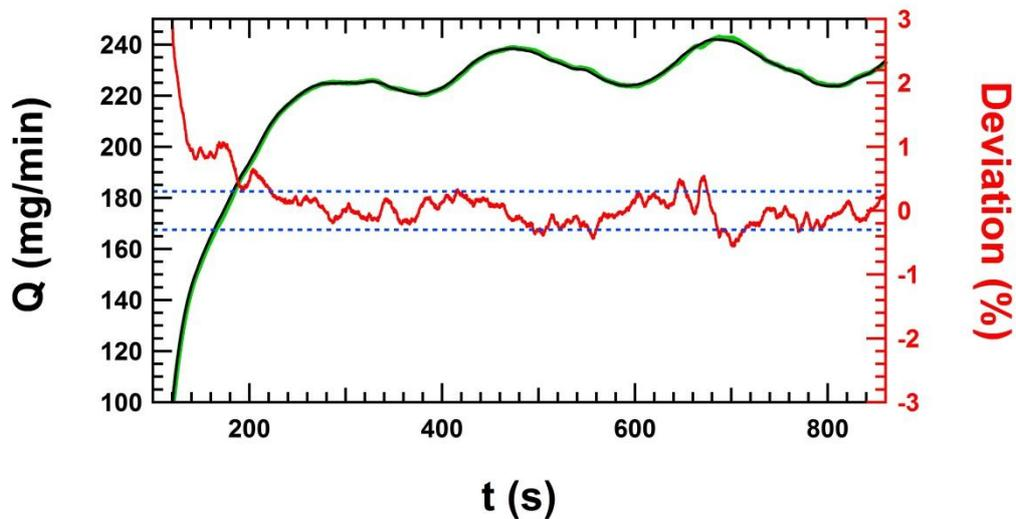
**Figure 29, DTI-Setup:** The instantaneous flow rate determined by the dynamic gravimetric method for a fit window of 20 s (left axis, green line) and the signal from the flow meter averaged over 20 s (left axis, black line) as well as the instantaneous deviation (right axis, red line). The dashed blue line is the stated uncertainty for the instantaneous flow rate (right axis).
