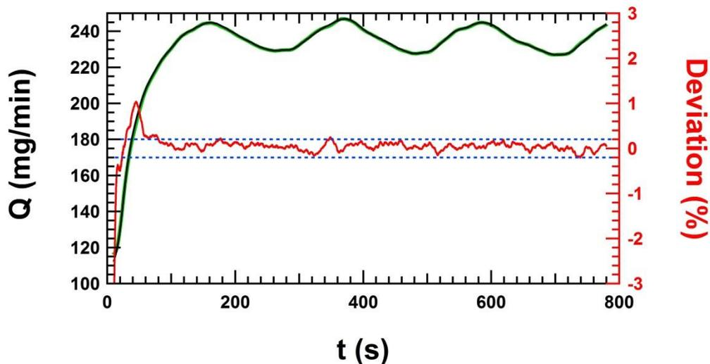
**Figure 18, METAS-Setup:** The instantaneous flow rate determined by the dynamic gravimetric method for a fit window of 20 s (left axis, green line) and the signal from the flow meter averaged over 20 s (left axis, black line) as well as the instantaneous deviation (right axis, red line). The dashed blue line is the stated uncertainty for the instantaneous flow rate (right axis).
