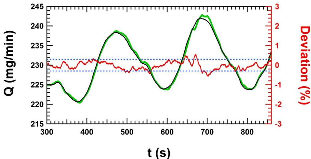
**Figure 31, DTI-Setup:** The instantaneous flow rate determined by the dynamic gravimetric method for a fit window of 20 s (left axis, green line) and the signal from the flow meter averaged over 20 s (left axis, black line) as well as the instantaneous deviation (right axis, red line). The dashed blue line is the stated uncertainty for the instantaneous flow rate (right axis). Only the data after the stabilization time are shown.
