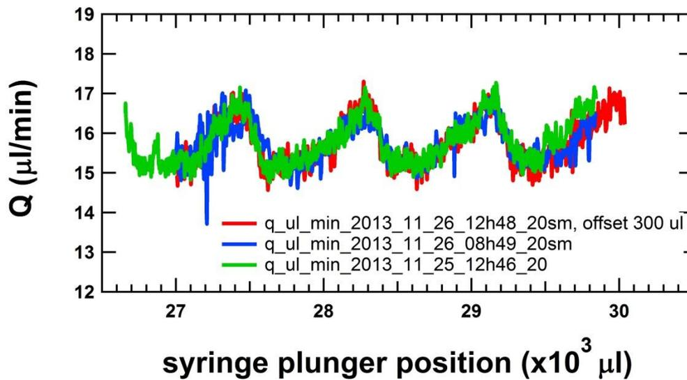
**Figure 12, METAS-Setup:** Instantaneous flow rates as a function of the position of the syringe plunger where a fit window of 20 s was used for the flow rate determination. 3 measurements were performed with the wet syringe (wet marked). The data of «2013\_11\_26\_12h48» are shifted with an offset of 300 µl in order to get an overlap of the pulsating flow pattern.
