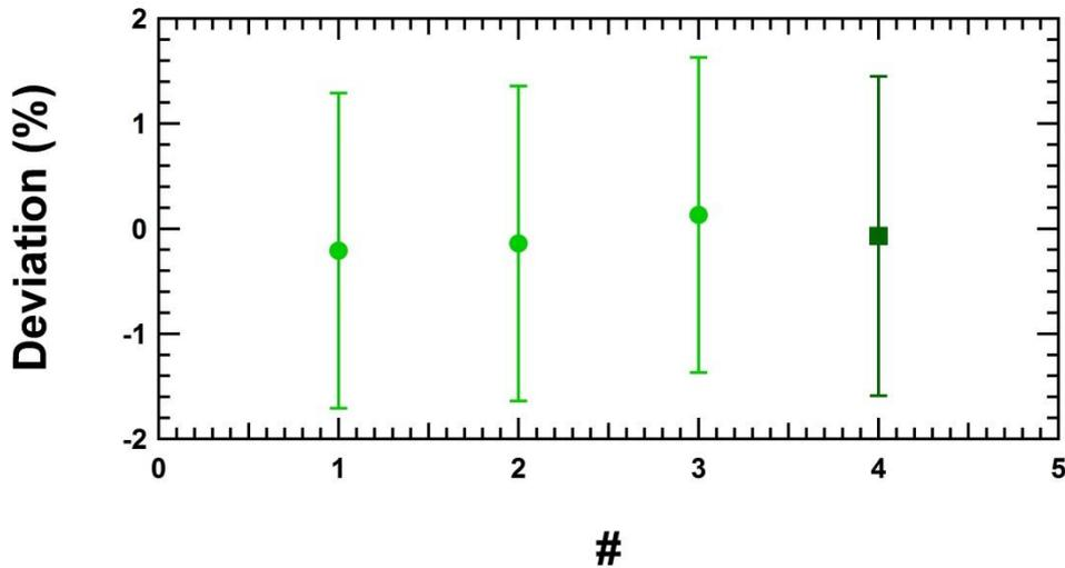
**Figure 27, DTI-Setup:** Deviations of the syringe pump using a wet syringe  $Q \sim 0.9$  ml/h (15.6  $\mu$ l/min). The square is the mean value of the 3 single points (circles).
