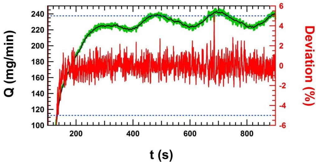
**Figure 28, DTI-Setup:** The instantaneous flow rate determined by the dynamic gravimetric method for a fit window of 3 s (left axis, green line) and the signal from the flow meter averaged over 3 s (left axis, black line) as well as the instantaneous deviation (right axis, red line). The dashed blue line is the stated uncertainty for the instantaneous flow rate (right axis).
