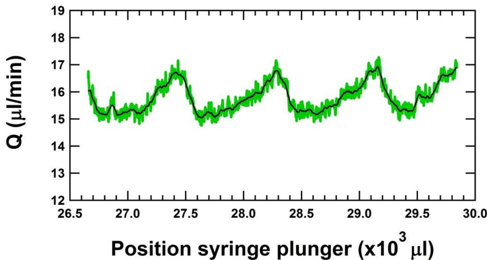
**Figure 14, METAS-Setup:** the original data of «2013\_11\_25\_12h46» (green line) and the smoothed curve which was averaged over 200 points corresponding to 52  $\mu\text{l}$  (black line).
