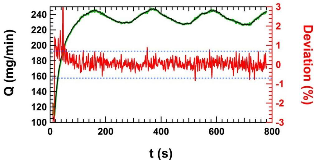
**Figure 17, METAS-Setup:** The instantaneous flow rate determined by the dynamic gravimetric method for a fit window of 3 s (left axis, green line) and the signal from the flow meter averaged over 3 s (left axis, black line) as well as the instantaneous deviation (right axis, red line). The dashed blue line is the stated uncertainty for the instantaneous flow rate (right axis).
