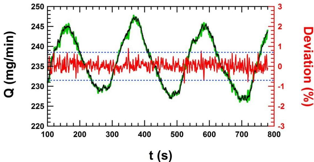
**Figure 19, METAS-Setup:** The instantaneous flow rate determined by the dynamic gravimetric method for a fit window of 3 s (left axis, green line) and the signal from the flow meter averaged over 3 s (left axis, black line) as well as the instantaneous deviation (right axis, red line). The dashed blue line is the stated uncertainty for the instantaneous flow rate (right axis). Only the data after the stabilization time are shown.
