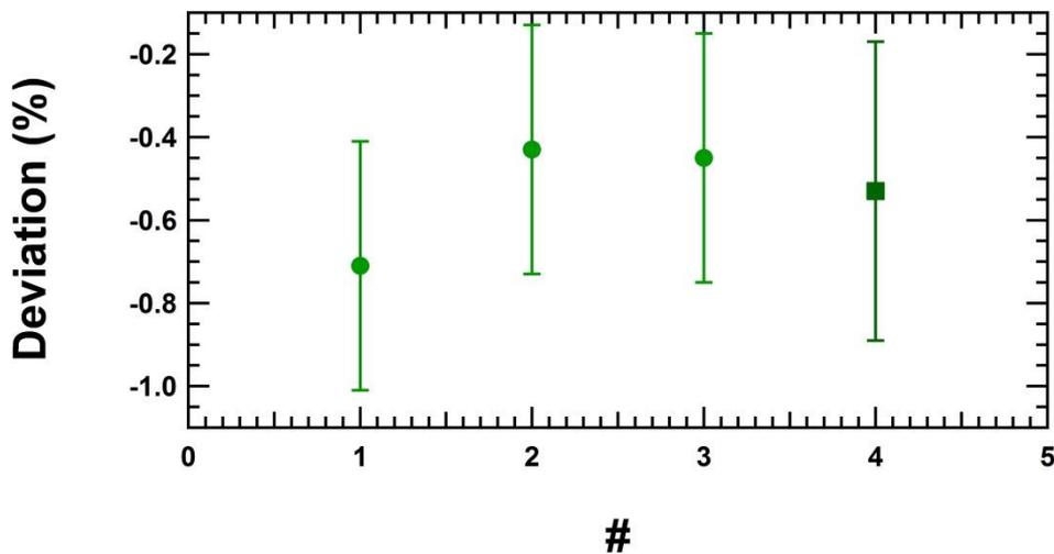
**Figure 24, DTI-Setup:** Deviations of the syringe pump using a syringe (wet marked, green circles) at  $Q \sim 14 \text{ ml/h}$  ( $233 \mu\text{l}/\text{min}$ ). The squares are the mean values of the 3 single points.
