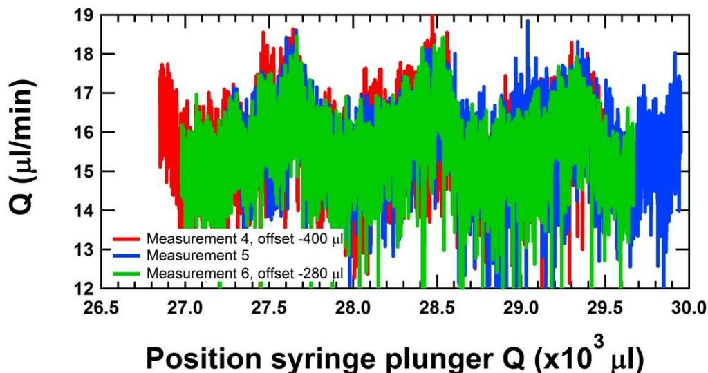
**Figure 26, DTI-Setup:** Instantaneous flow rates as a function of the position of the syringe plunger where a fit window of 20 s was used for the flow rate determination. 3 measurements were performed with the syringe (wet marked). The data are shifted with an offset in order to get an overlap of the pulsating flow pattern.
