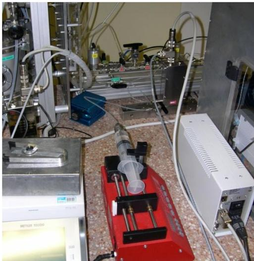
**Figure 5, METAS-Setup:** The Coriolis flow meter is connected downstream of the syringe pump and to the micro flow facility at METAS.
