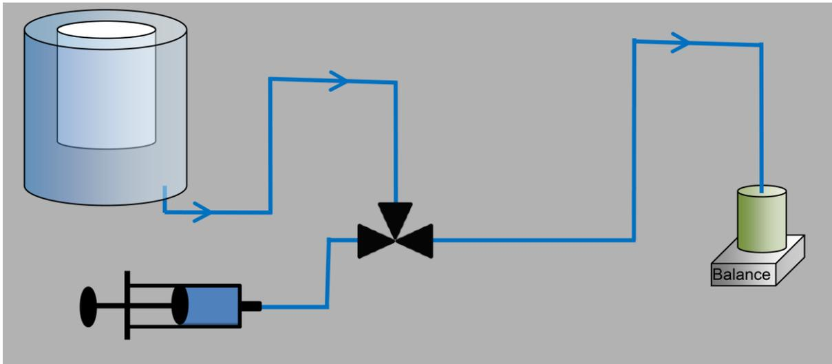
**Figure 2, METAS-Setup:** The syringe pump is connected to the micro flow facility with its gravimetric method to determine the volume flow rate generated by the syringe pump (micro flow facility METAS).
