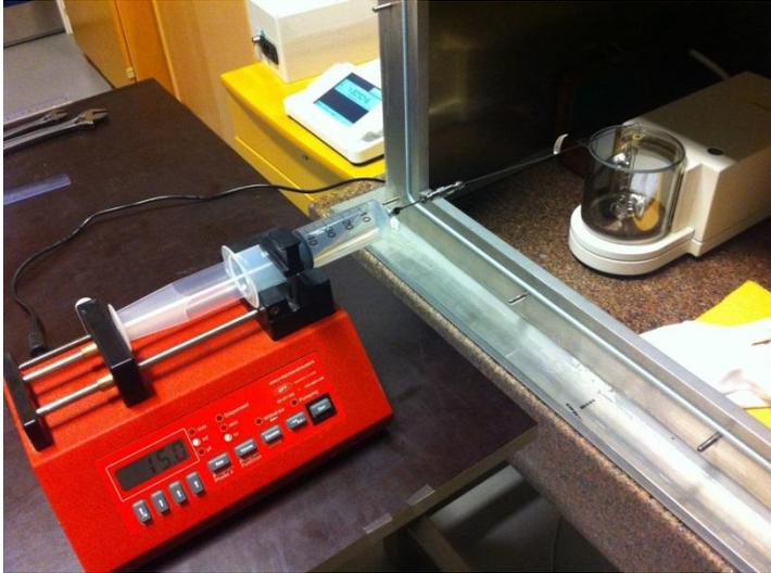
**Figure 6, DTI-Setup:** The syringe pump is connected to the micro flow facility at DTI.
