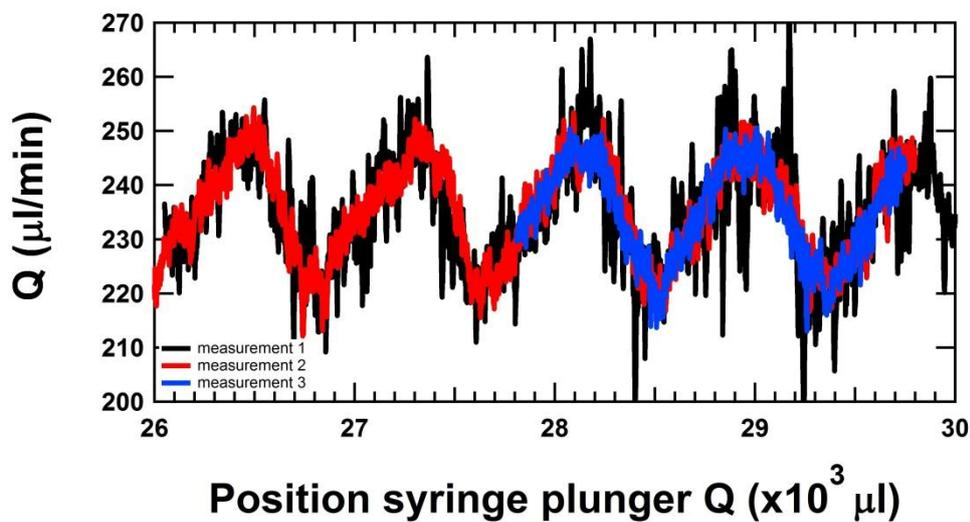
**Figure 22, DTI-Setup:** Instantaneous flow rates as a function of the position of the syringe plunger where a fit window of 3 s was used for the flow rate determination. Details of the different curves can be found in Table 15.
