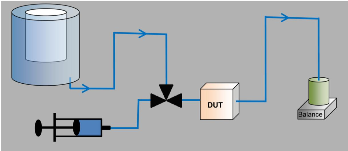
**Figure 4, METAS-Setup:** The «inlet» of the syringe pump is connected to the water reservoir and the «outlet» is connected to the coriolis flow meter which is then connected to the piping leading to the beaker on the balance (micro flow facility METAS).
