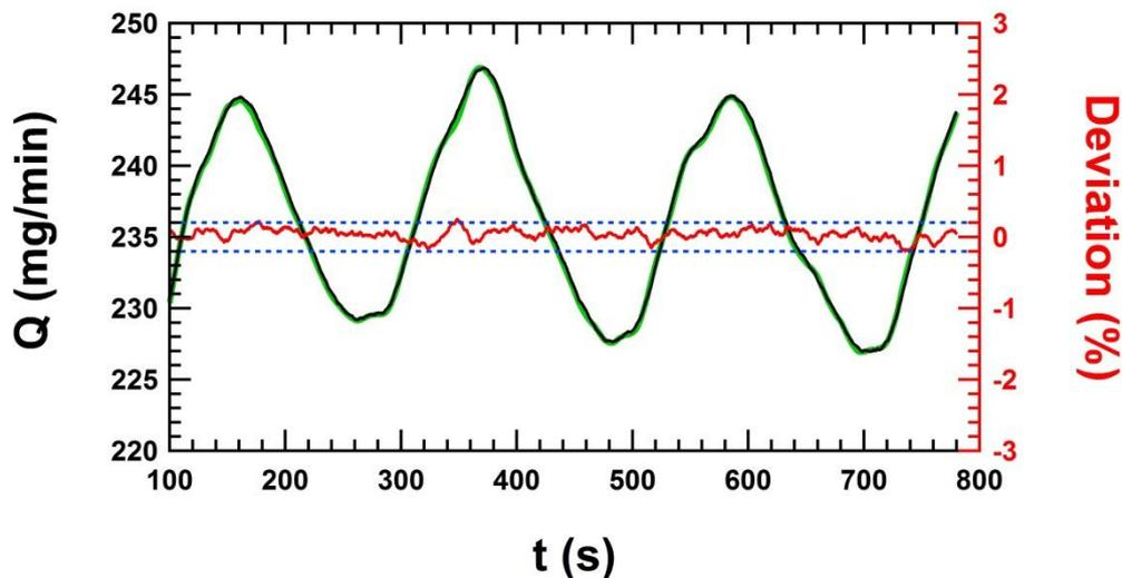
**Figure 20, METAS-Setup:** The instantaneous flow rate determined by the dynamic gravimetric method for a fit window of 20 s (left axis, green line) and the signal from the flow meter averaged over 20 s (left axis, black line) as well as the instantaneous deviation (right axis, red line). The dashed blue line is the stated uncertainty for the instantaneous flow rate (right axis). Only the data after the stabilization time are shown.
