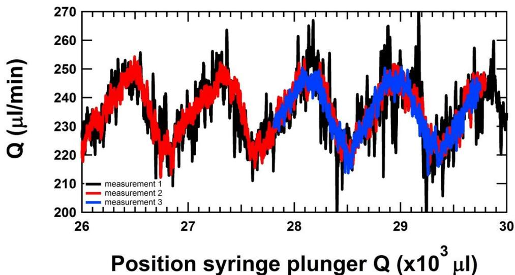
**Figure 23, DTI-Setup:** Instantaneous flow rates as a function of the position of the syringe plunger where a fit window of 20 s was used for the flow rate determination. Details of the different curves can be found in Table 15.
