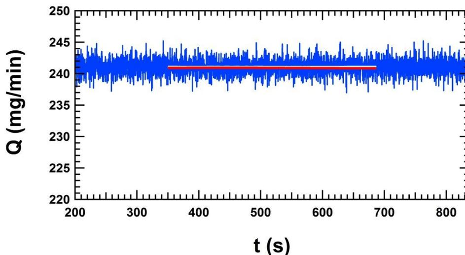
**Figure 15, METAS-Setup:** raw data of the M12P (blue line), the averaged data of the M12P (cyan line) and the averaged data of the reference flow rate of the experiment «2013\_12\_02\_14h48» (red line). The fit window and the averaging time is 300 s.
