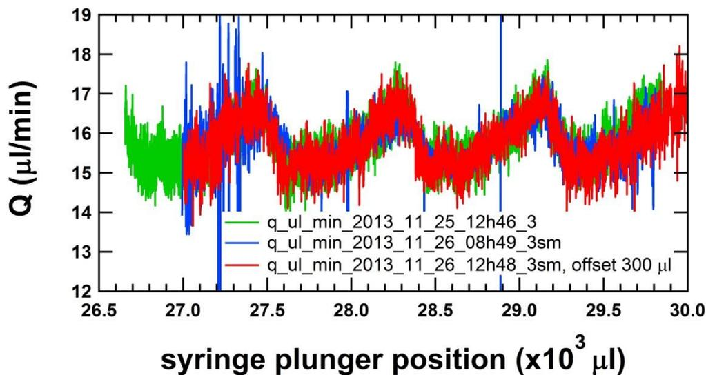
**Figure 11, METAS-Setup:** Instantaneous flow rates as a function of the position of the syringe plunger where a fit window of 3 s was used for the flow rate determination. 3 measurements were performed with the wet syringe (wet marked). The data of «2013\_11\_26\_12h48» are shifted with an offset of  $300 \mu\text{l}$  in order to get an overlap of the pulsating flow pattern.
