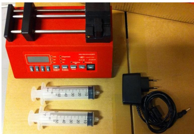
**Figure 1:** The Syringe pump consisting of the syringe driver Aladdin-300 with its power supply and 2 syringes of 60 ml. One is marked with “dry” (not used) and the other is marked with “wet” (first use at DTI).
