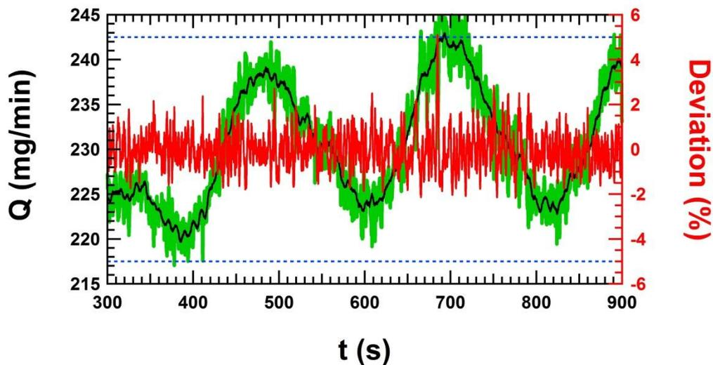
**Figure 30, DTI-Setup:** The instantaneous flow rate determined by the dynamic gravimetric method for a fit window of 3 s (left axis, green line) and the signal from the flow meter averaged over 3 s (left axis, black line) as well as the instantaneous deviation (right axis, red line). The dashed blue line is the stated uncertainty for the instantaneous flow rate (right axis). Only the data after the stabilization time are shown.
