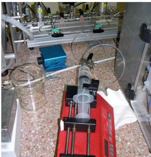
**Figure 3, METAS-Setup:** The syringe pump is connected to the micro flow facility at METAS.
