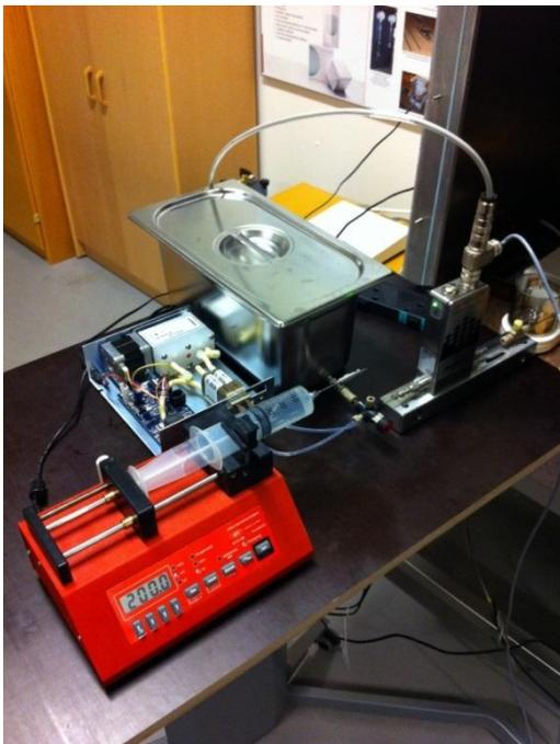
**Figure 7, DTI-Setup:** The Coriolis flow meter is connected downstream of the syringe pump and to the micro flow facility at DTI.
