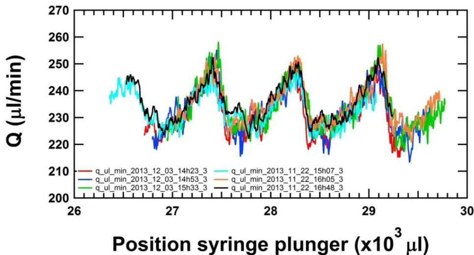
**Figure 8, METAS-Setup:** Instantaneous flow rates as a function of the position of the syringe plunger where a fit window of 3 s was used for the flow rate determination. Using 2 syringes 6 measurements were performed. Details of the different curves can be found in Table 5.
