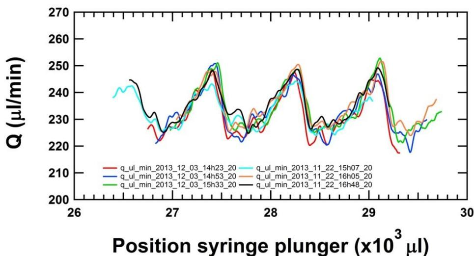
**Figure 9, METAS-Setup:** Instantaneous flow rates as a function of the position of the syringe plunger where a fit window of 20 s was used for the flow rate determination. Using 2 syringes 6 measurements were performed. Details of the different curves can be found in Table 5.
