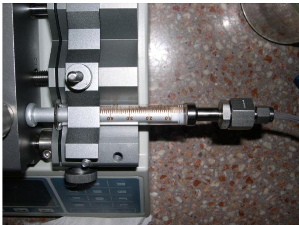
Figure 16: syringe (5000 \mu\text{l} volume) mounted in the syringe pump.
