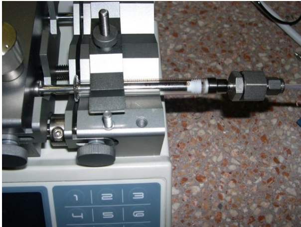
Figure 13: syringe (2500 \mu\text{l} volume) mounted in the syringe pump.
