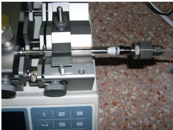
Figure 9: syringe (2500 \mu\text{l} volume) mounted in the syringe pump.
