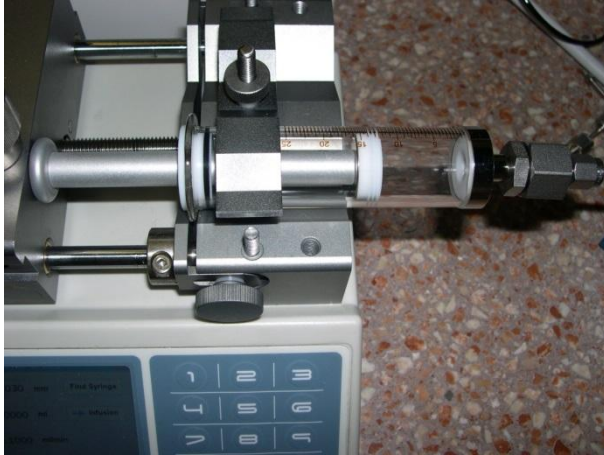
Figure 23: syringe (25000 \mu\text{l} volume) mounted in the syringe pump.
